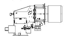
DN 100 gas connection from the side Elbow100/100 adapter already included as standard equipment
