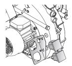
To measure the burner working time a hours counter kit is available.
