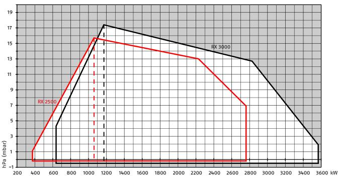
Please note: it is important to be aware that in order to achieve an ULTRA low NOx emission performance, it is required to work with a high excess air; as consequence the combustion chamber back pressure could increase up to roughly 30% more.
