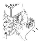
The seal control function is included on Burner Digital Management System, it is only necessary to add the PVP kit on the gas train.
