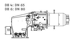
DN 65 gas connection from below Elbow adapter DN 65 required DN 80 gas connection from below (for gas versions). Elbow adapter DN 80 required.
