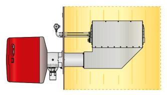
**L1 -** Angle configuration with combustion head developed in horizontal in primary air duct
