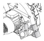
To measure the burner working time a hours counter kit is available.
