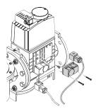
The seal control function is included on Burner Digital Management System, it is only necessary to add the PVP kit on the gas train.
