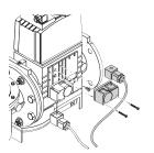
The seal control function is included on Burner Digital Management System, it is only necessary to add the PVP kit on the gas train.
