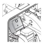
To have 20 s ventilation after opening of thermostats chain, a special kit is available.
