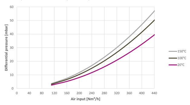
Pressure drop shall be taken between pressure Tap B and C
