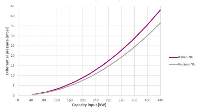
Pressure drop shall be taken as differential between pressure Tap A and B
