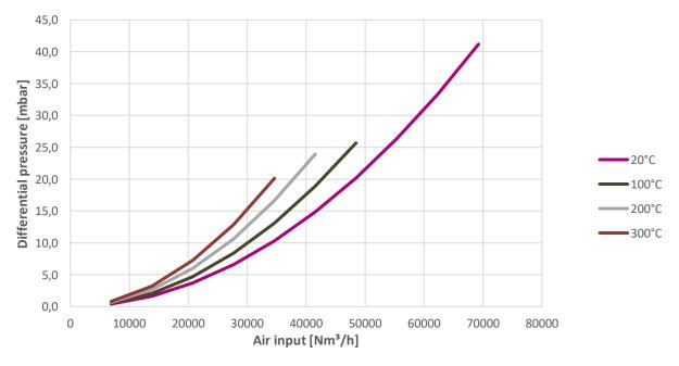
Pressure drop should be taken between the chamber and windbox pressure tap (tap B)
