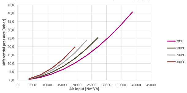
Pressure drop should be taken between the chamber and windbox pressure tap (tap B)
