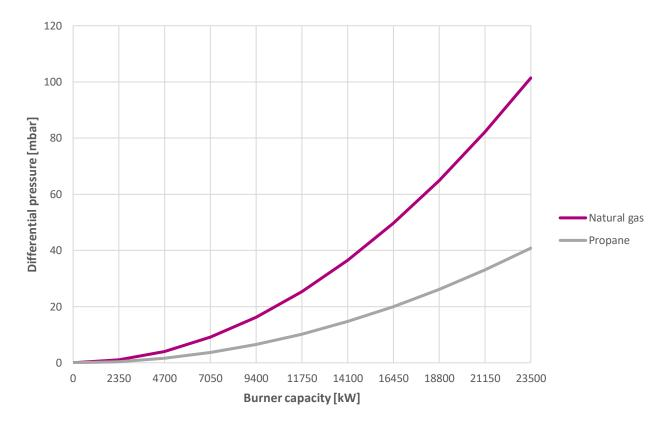
Note: Pressure drop curves should be used as a guide for setting up burner. It is recommended to use fuel flow measurements for determining actual fuel flows.
