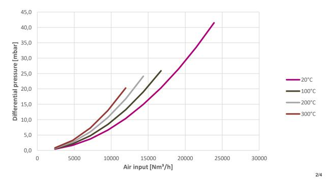
Pressure drop should be taken between the chamber and windbox pressure tap (tap B)
