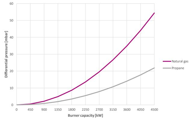
Pressure drop should be taken as differential between the chamber and gas gun pressure tap A.
