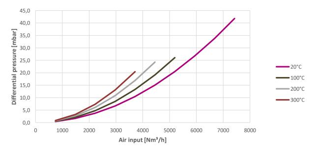
Pressure drop should be taken between the chamber and windbox pressure tap (tap B)
