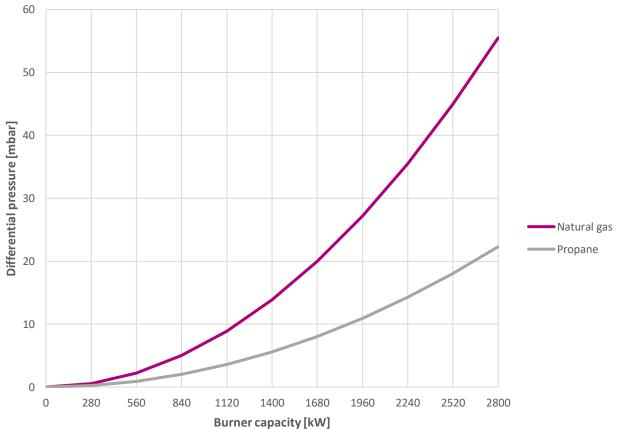
Note: Pressure drop curves should be used as a guide for setting up burner. It is recommended to use fuel flow measurements for determining actual fuel flows.
