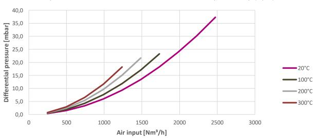
Pressure drop should be taken between the chamber and windbox pressure tap (tap B)
