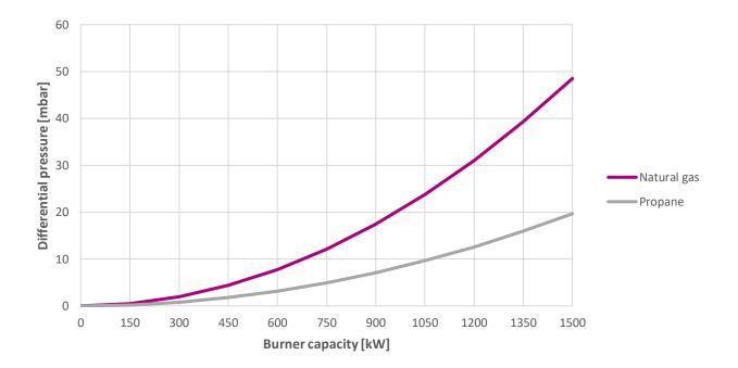
Note: Pressure drop curves should be used as a guide for setting up burner. It is recommended to use fuel flow measurements for determining actual fuel flows.
